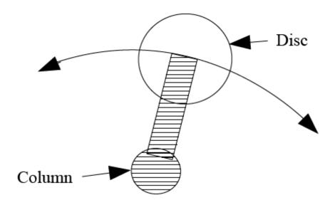
This diagram above shows the pick arm holding a disc, viewed from above. The Disc arrowed line shows the potential adjustment direction which can be achieved from the keypad controlled positioning of the pick arm.
